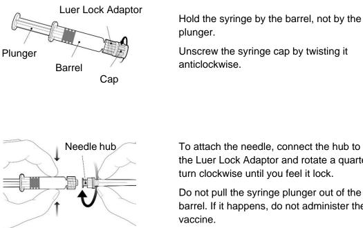
Unscrew the syringe cap by twisting it
