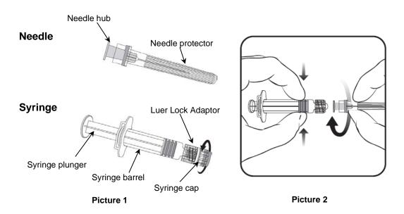
Always hold the syringe by the barrel, not by the syringe plunger or the Luer Lock Adaptor (LLA), and maintain the needle in the axis of the syringe (as illustrated in picture 2). Failure to do this may cause the LLA to become distorted and leak.
